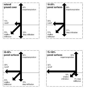
Figure 8: Impacts of Impervious Surfaces
