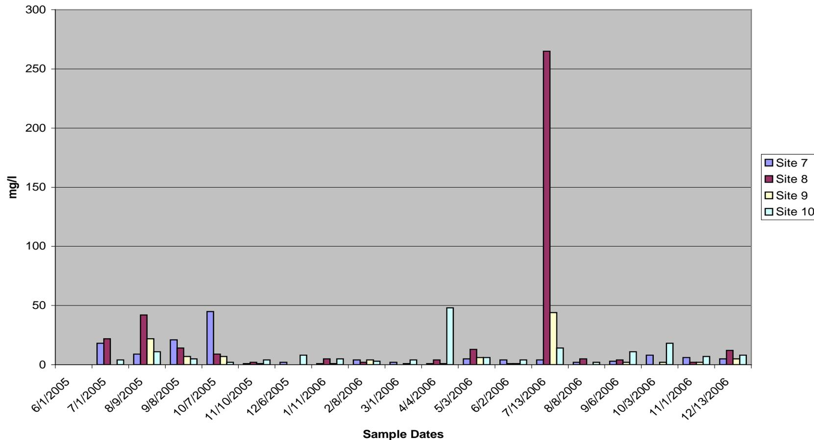
Figure 69: Graphical depiction of total suspended solids for test sites 7 through 10. The Y axis represents milligrams per liter of water.
