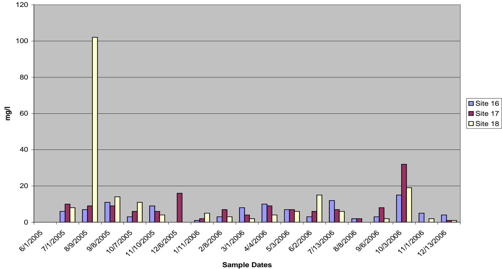
Figure 72: Graphical depiction of total suspended solids for test sites 16 through 18. The Y axis represents milligrams per liter of water.
