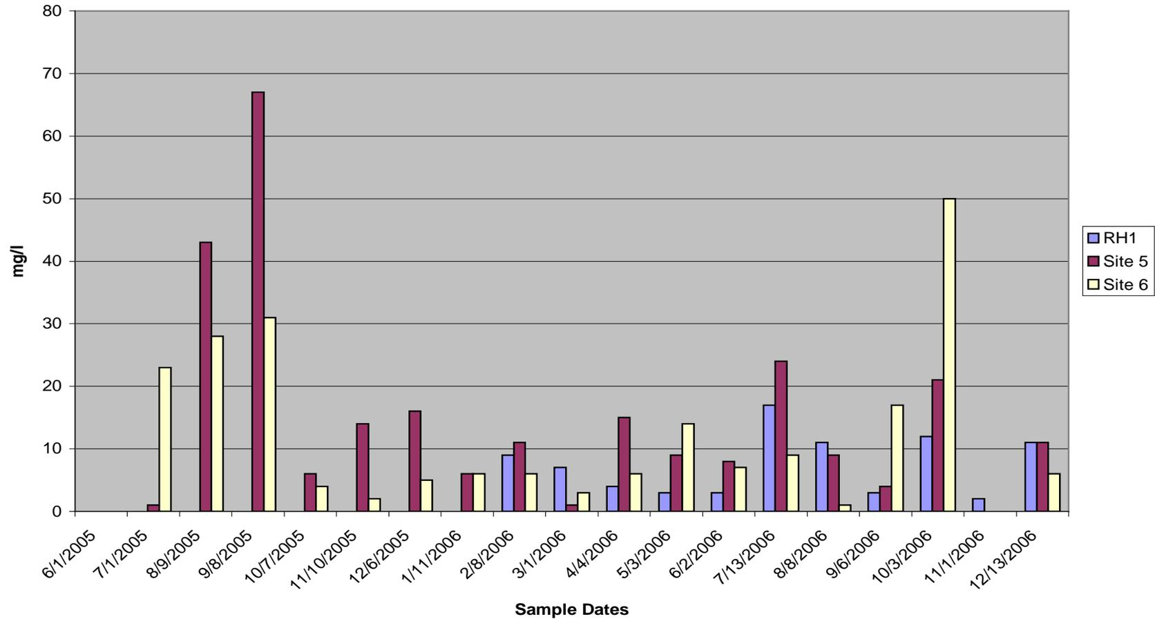
Figure 68: Graphical depiction of total suspended solids for test sites RH1 through 6. The Y axis represents milligrams per liter of water.
