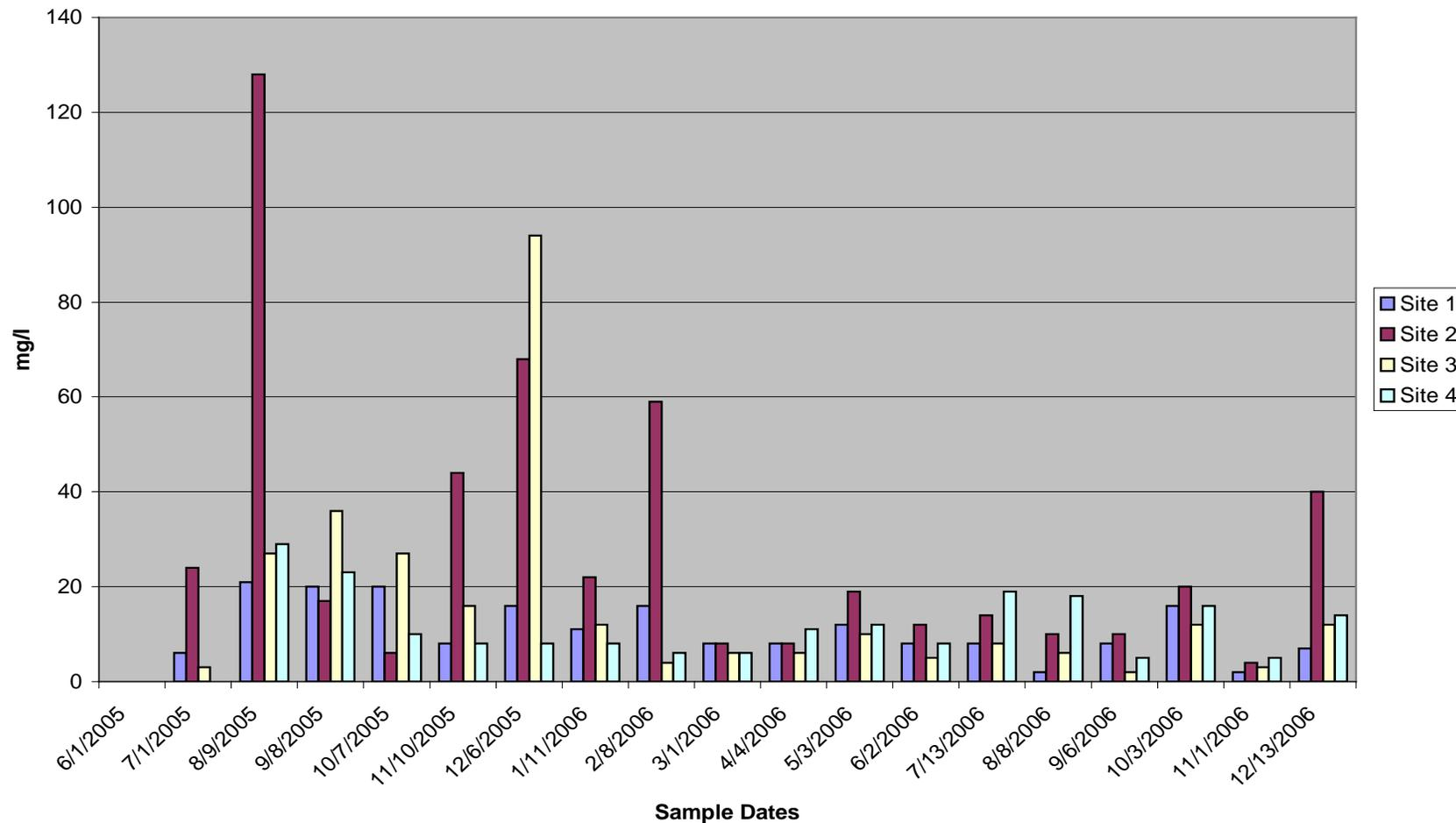
Figure 67: Graphical depiction of total suspended solids for test sites 1 through 4. The Y axis represents milligrams per liter of water.
