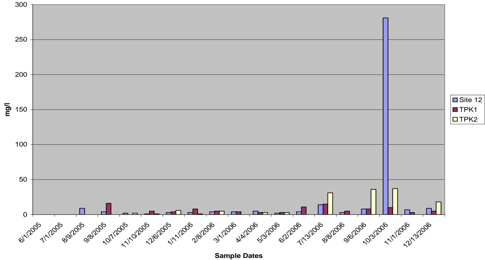
Figure 70: Graphical depiction of total suspended solids for test sites 12 through TPK2. The Y axis represents milligrams per liter of water.
