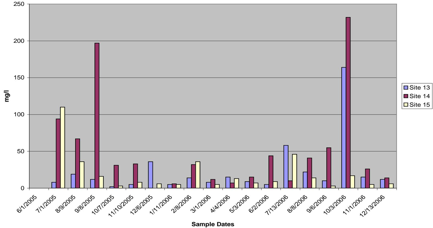
Figure 71: Graphical depiction of total suspended solids for test sites 13 through 15. The Y axis represents milligrams per liter of water.
