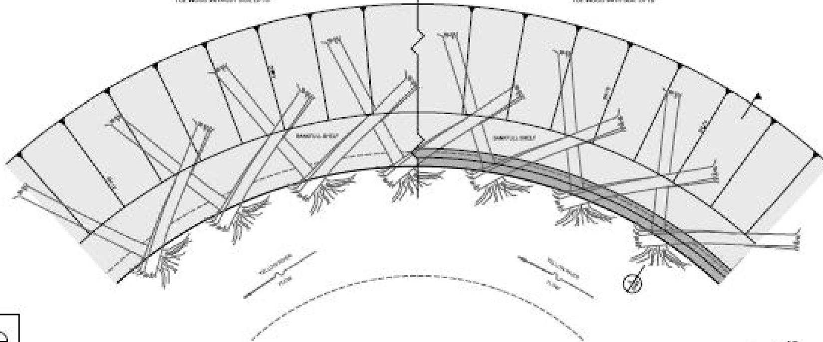
1 PLAN VIEW - TOE WOOD AND SOIL LIFTS
